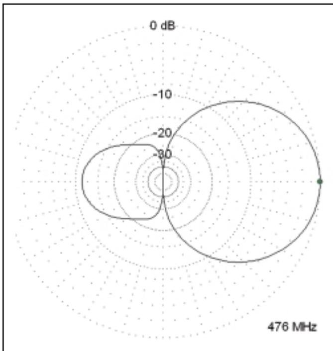
Figure 1. EZ HDTV pattern on UHF TV Channel 14.
