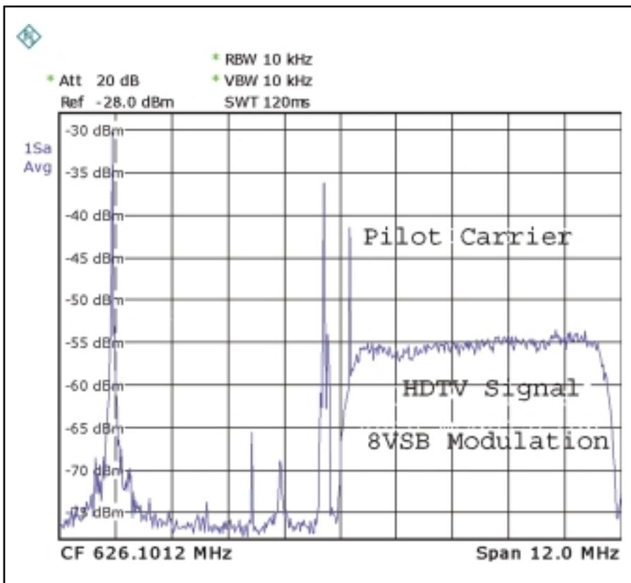
Figure 7. Side-by-side analog NTSC and digital 8VSB.
