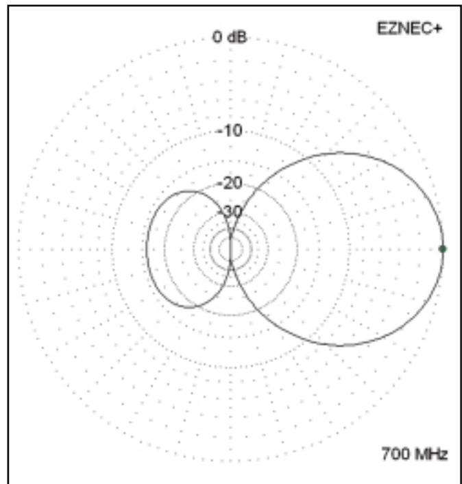
Figure 2. EZ HDTV pattern on UHF TV Channel 52.
